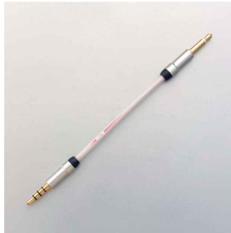
coxc_01_3432 3.5 4p - 3.5 2p silver plated PCOCC foamed PE insulation aluminum tape + copper shield pvc jacket gold plated plug aluminum sleeve length:0.1m jan:4534165012685
