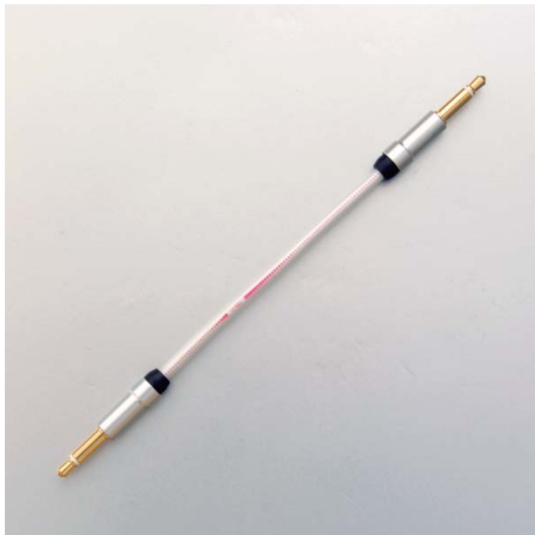
coxc_01_3232 3.5 2p - 3.5 2p silver plated PCOCC foamed PE insulation aluminum tape + copper shield pvc jacket gold plated plug aluminum sleeve length:0.1m jan:4534165012661
